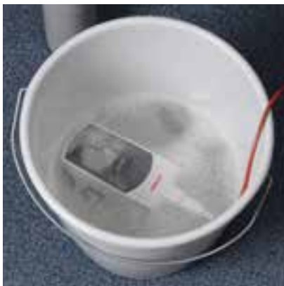
TF 410 - still working, thanks to IP67
