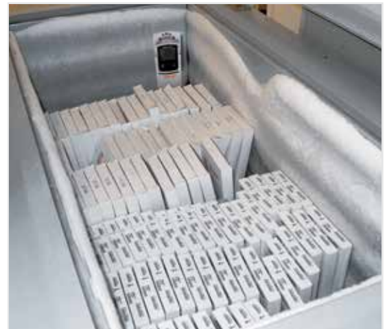
The use of digital data loggers (such as ebro EBI 300 series) to monitor temperature changes along the vaccine cold chain is vital to the vaccines' effectiveness. 使用數字數據記錄器（例如 ebro EBI 300 系列）來監測疫苗冷鏈中的溫度變化對於疫苗的有效性至關重要。
